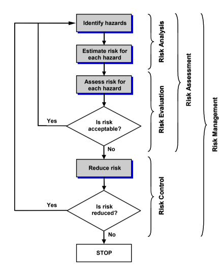
Typical Procedure for Risk Analysis, Evaluation and Control acceptable levels by design measures, then risks should be brought to an acceptable level through mitigation efforts such as process qualification.
