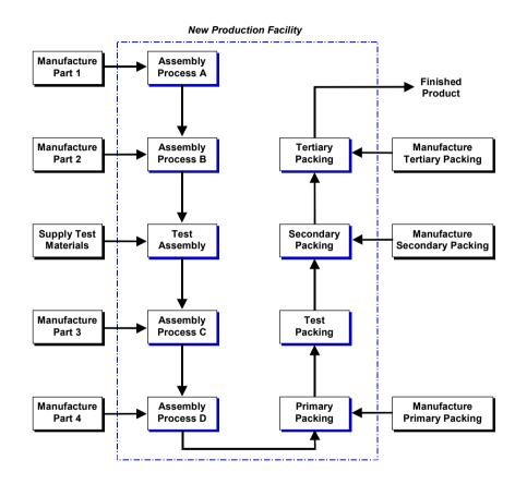
**Example of a Process Flow Diagram**
