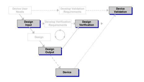
Exploring the Effects of Process Re-design Using the DFV V-Model In order to understand the influences of process re-design on the device, the designer must explore the impacts on device design input, design output, design verification and the entire device validation. This is shown in terms of the Design for Validation V-Model on the adjacent diagram.
