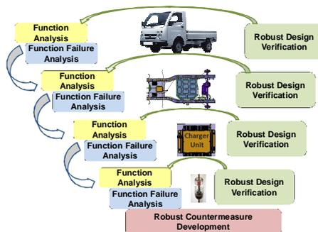
Figure 4.10. SED framework based on FMA
