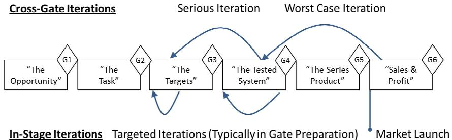
**Figure 10.5.** In-stage and cross-gate iterations
