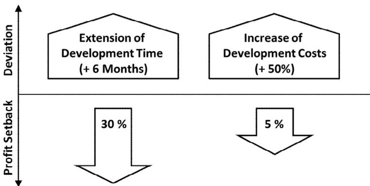
**Figure 10.6.** Profit setback caused by an extension of development time and an increase of development cost (product life time: 5 years) according to Hall and Jackson (1992)
