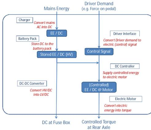
**Figure 4.3.** System state flow diagram for an electric vehicle powertrain (EVP) system
