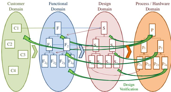
**Figure 4.2.** Functional decomposition by mapping and zigzagging between customer, function, design and process domains
