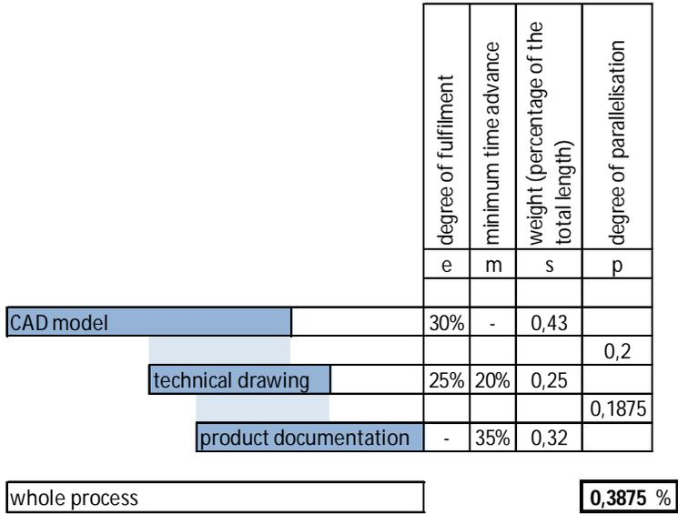
Figure 6.8. Sample data for the calculation of the degree of parallelisation
