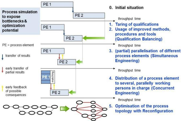
**Figure 6.6.** Stages of process optimisation (Schabacker and Vajna, 2003)
