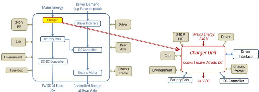
**Figure 4.11.** Illustration of the cascade of interfaces to subsystem level
