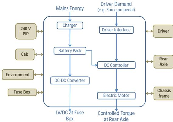
Figure 4.5. System boundary diagram for the EVP system
