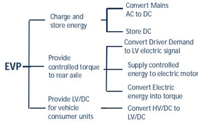
Figure 4.4. Function tree for the EVP system
