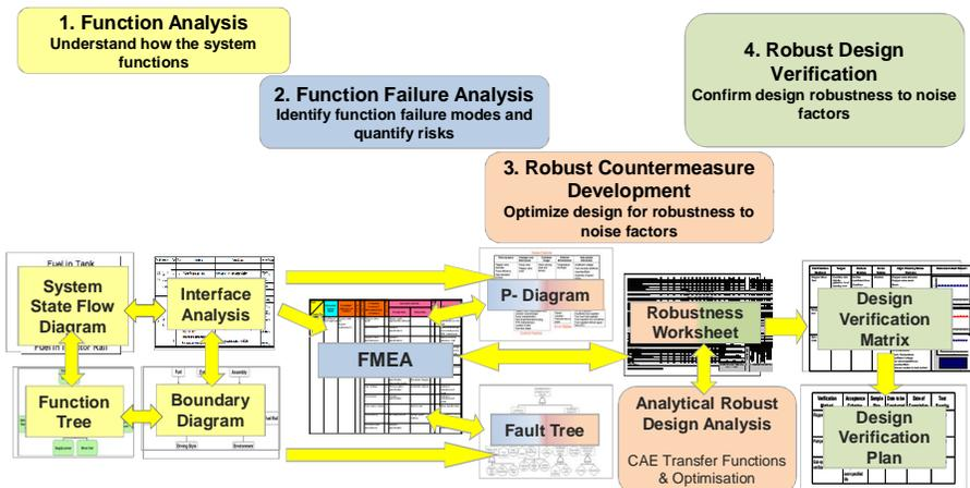
Figure 4.1. FMA framework, showing process steps and support tools
