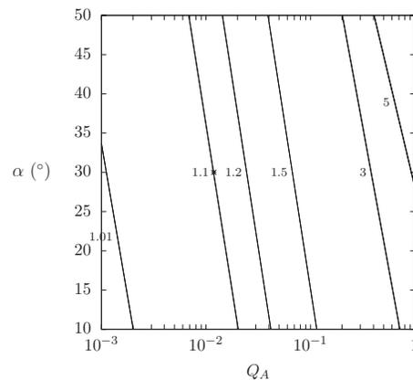
Fig. 6 Friction law A: contours of  $R_{\text{out}}^{\text{lim}}$  in the  $(\alpha, Q_A)$  plane, the star marks the working point of a typical low-grade sugar continuous centrifuge
