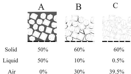
Fig. 2 Microstructure and volume fraction of the solid/liquid/air phases at stations A, B, and C
