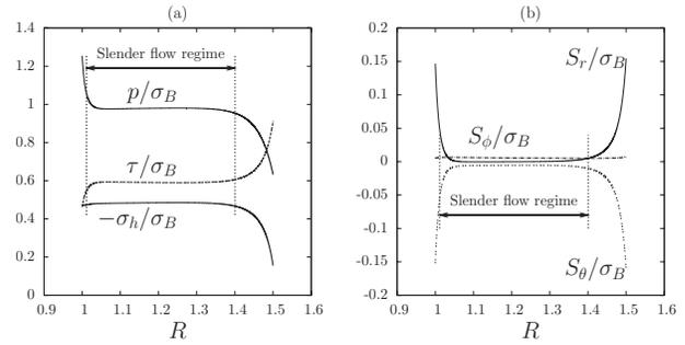
**Fig. 11 Model B nondimensional stresses: (a) hydrostatic stress  $\sigma_h$  and wall traction  $(\tau, p)$  (b) direct components of the deviatoric stress tensor,  $\alpha=30$  deg,  $\hat{b}=0.9$ ,  $\hat{\mu}=10^{-1}$ ,  $Q_B=10^{-2}$ , and  $R_{out}=1.5$**
