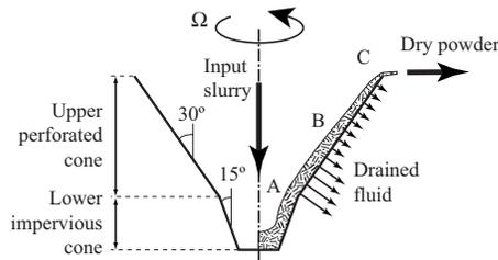
Fig. 1 Cross-section of a typical conical centrifugal filter
