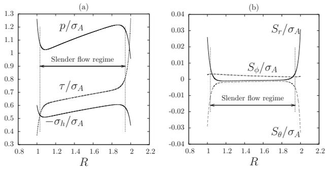
**Fig. 7 Friction law A: dimensionless stresses for  $\alpha=30$  deg,  $Q_A=0.1$ , and  $R_{out}=2$ . (a) Hydrostatic stress  $\sigma_h$  and wall traction  $(\tau, p)$  and (b) direct components of the deviatoric stress tensor.**
