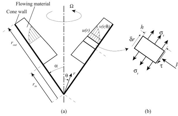
**Fig. 3** (a) Cone geometry and (b) element of material of thickness  $h$  and of infinitesimal radial thickness  $\delta r$
