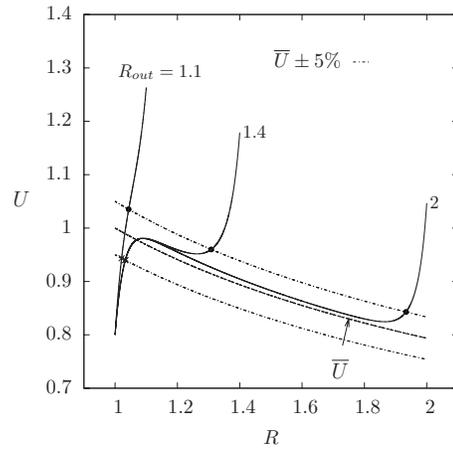
Fig. 5 Friction law A: solutions for various values of  $R_{\text{out}}$  compared with  $\bar{U}$  with  $\alpha = 30$  deg and  $Q_A = 0.1$
