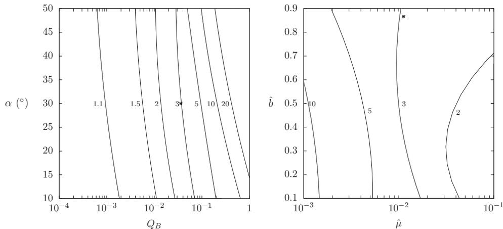
**Fig. 10 Model B: Limit radius  $R_{out}^{lim}$  linearized contours versus (a)  $Q_B$  and  $\alpha$  and (b)  $\hat{\mu}$  and  $\hat{b}$  with the appropriate parameters held constant at  $\alpha=30$  deg,  $\hat{b}=0.87$ ,  $\hat{\mu}=1.1 \times 10^{-2}$ ,  $P_B=4.4 \times 10^{-2}$ , and  $Q_B=3.6 \times 10^{-2}$ . The star on each map marks the working point of a typical low-grade sugar continuous centrifuge.**
